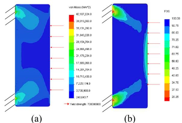
Fig. 15 (a) Von mises stress of quartz. (b) safety factor of quartz
