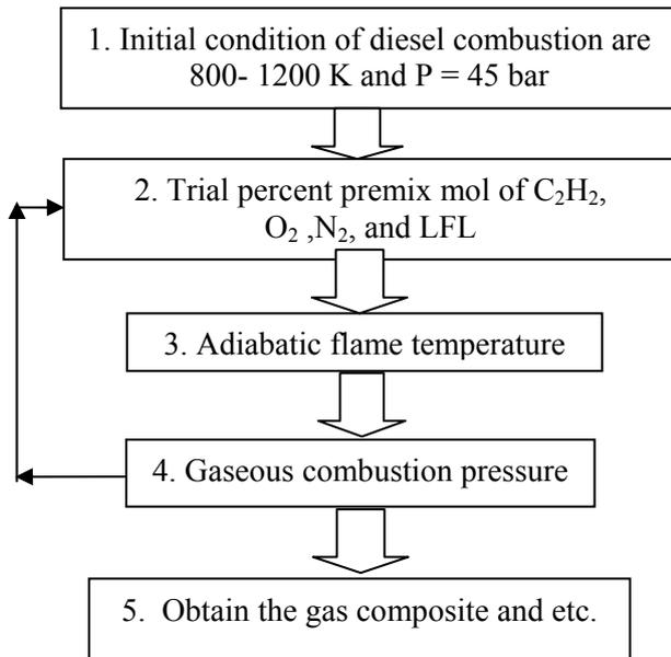
Fig. 3 Procedure to achieve diesel combustion conditions with premix gas combustion.
