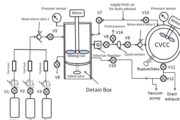
Fig. 9 Schematic gas supply system
