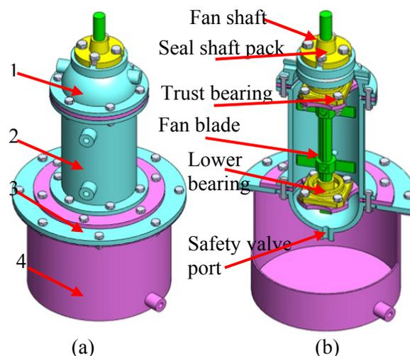
Fig 12 (a) Mixing tank layout (b) Section view of mixing tank and detail.
