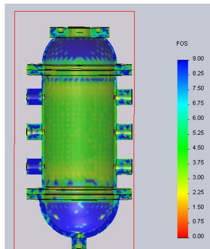
Fig. 11 Safety factor of mixing tank
