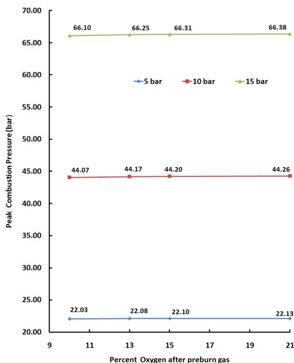
Fig. 7 Peak combustion pressure in different initial combustion pressure
