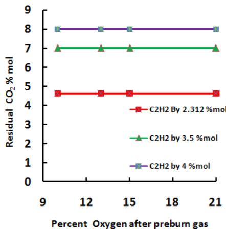
Fig. 4 Percent of CO<sub>2</sub> from various percent oxygen after pre-burn gas with different percent fraction of C<sub>2</sub>H<sub>2</sub>.
