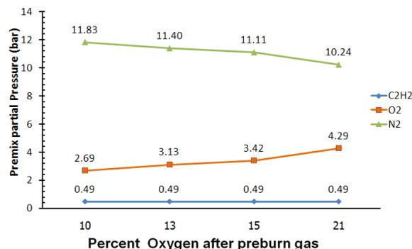
Fig. 8 Partial pressure of preburn gas composition with compressibility (Z) factor at different percent mol of O<sub>2</sub> concentration.
