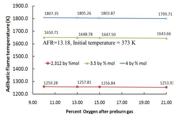
Fig.6 Adiabatic flame temperature with different percent of C<sub>2</sub>H<sub>2</sub> and percent of O<sub>2</sub> concentration after combustion.
