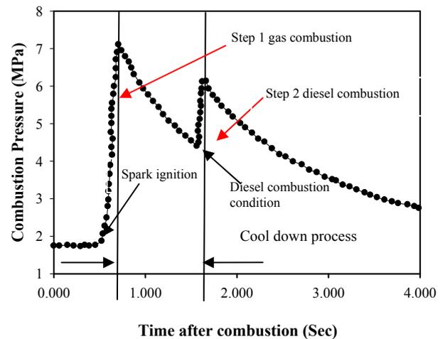
Fig.2 Historical pressure data of two stage combustion for simulated diesel combustion conditions. [6]
