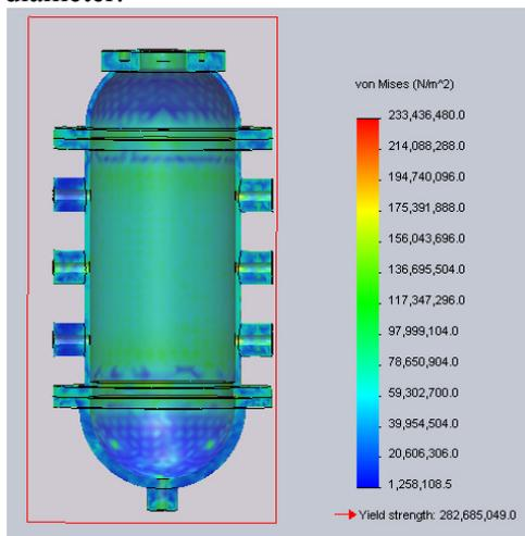
Fig 10 Von mises stress of mixing tank
