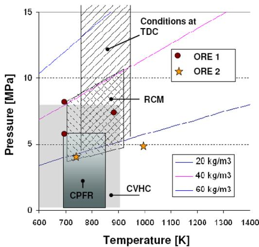
Fig.1 In cylinder condition during diesel injection conditions with different the optical tools [6].
