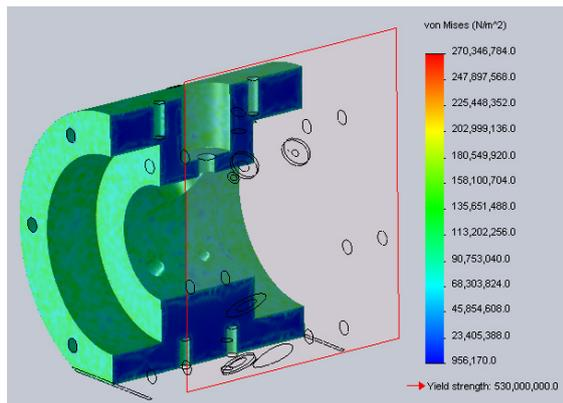
Fig. 13 Von mises stress of CVCC
