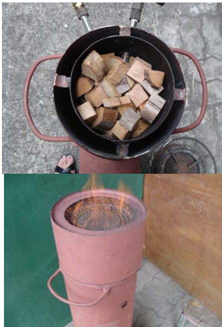
Fig.3 Flame feature from gasification of wood chip
