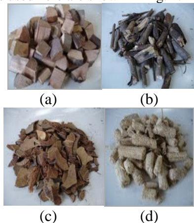
Fig 2. Biomass fuel used in the present study (a) wood chip of eucalyptus (b) wood twig (c) coconut shell and (d) corncob
