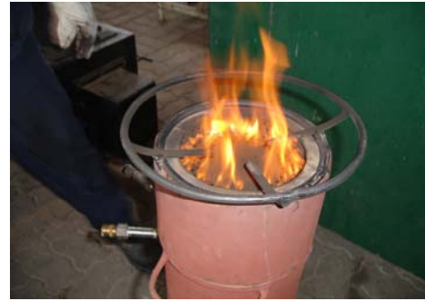
Fig. 5 Global flame feature from the gasification of coconut shell
