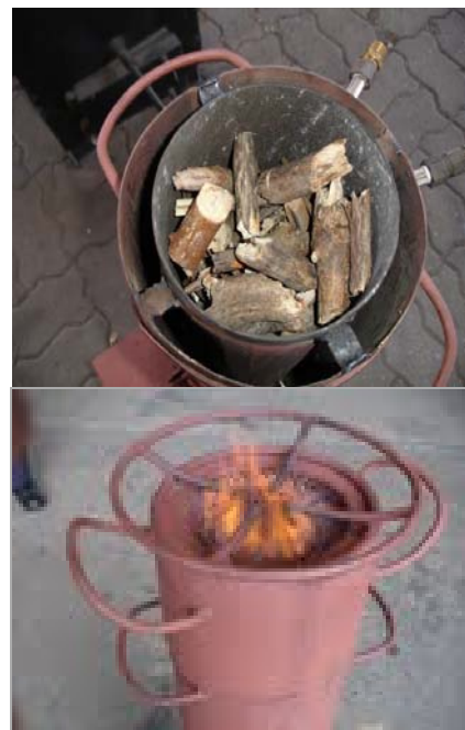
Fig. 4 Flame feature from gasification of wood twigs
