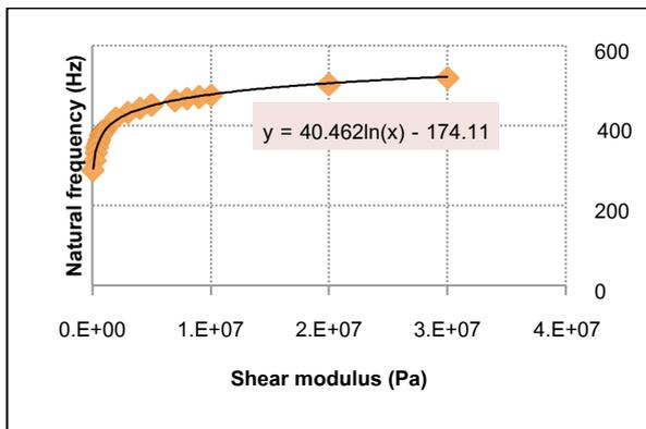
Fig. 12 First mode frequency and it's trend line equation of Experimental testing model varying Thin-layer's Shear modulus fixed Thin-layer thickness ratio = 1:30
