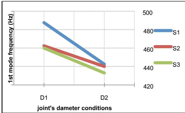
Fig. 11 First mode frequency of 8 joints plate (N3) with various joint's diameter conditions
