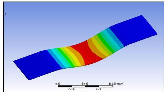
Fig.14 Mode shape deformation (first mode) from finite element method (blue zone:clamped area)
