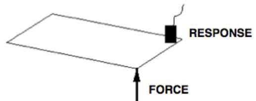
Fig. 2 Simple Plate Excitation/Response Model
