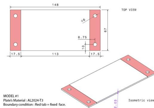
Fig. 5 Simple aluminum plate – PS440 dimension
