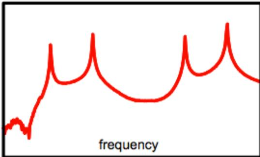
Fig. 3 Simple Plate Frequency Response Function
