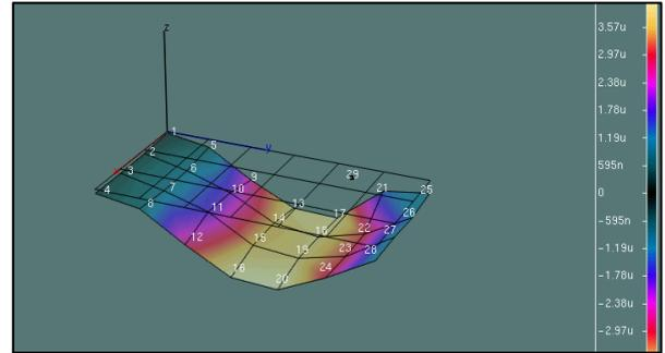
Fig.13 Mode shape deformation (first mode) from experiment
