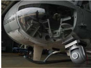
Fig.5 The gimbal mounted on the helicopter
