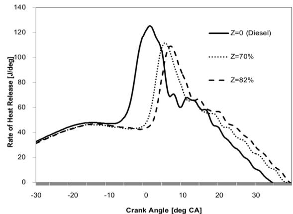
Fig. 7 Comparison of heat release rate between diesel and DDF at Z=0%, 70% and 82%
