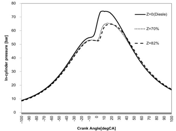
Fig. 6 Comparison of in-cylinder pressure between diesel and DDF at Z=0%, 70% and 82%
