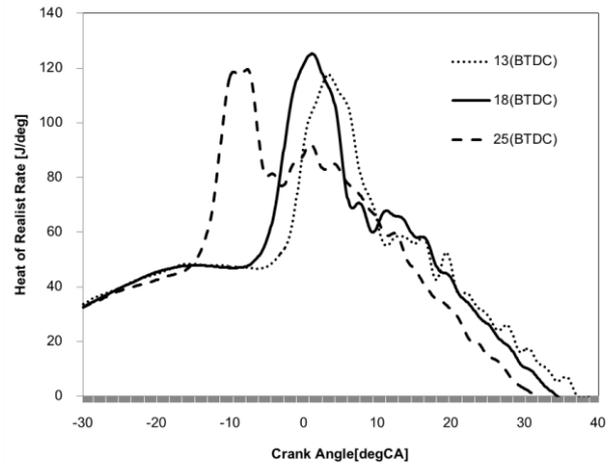
Fig. 5 Rate of heat release at injection timing 13,18 and 23 deg BTDC
