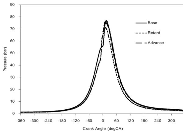
Fig. 4 In-cylinder pressure at injection timing 13,18 and 23 deg BTDC
