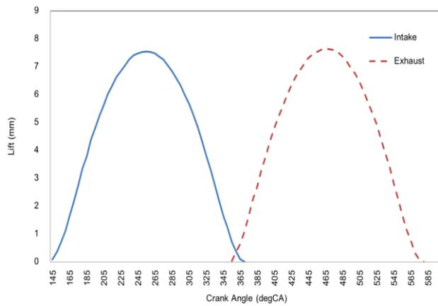
Fig. 3 Intake and exhaust valve curve for KUBOTA RT140
