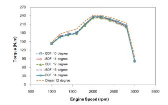
Figure 2 Engine Torque at full load with adjusted injection timings
