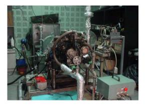
Figure 1 Experimental Setup A flame ionization detector (FID) analyser was used to measure exhaust UHC emissions.
