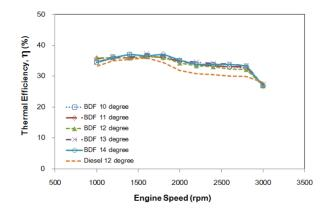
Figure 4 Thermal efficiency at full load with adjusted injection timings
