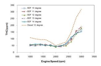
Figure 7 Total hydrocarbon emissions at full load with adjusted injection timings
