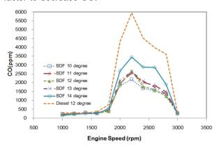
Figure 5 CO emissions at full load with adjusted injection timings
