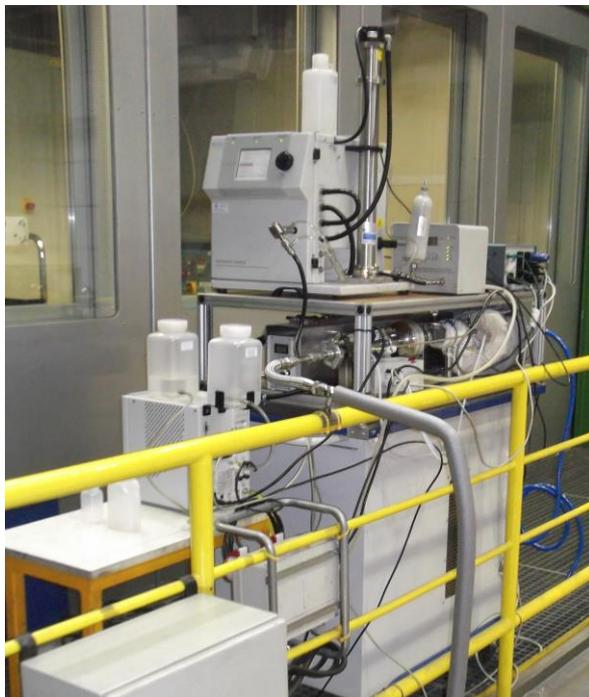
Fig. 3 A Scanning Mobility Particle Sizer (SMPS) for particle size distribution at “Institute for Internal Combustion Engines and Thermodynamics, Graz University of Technology.
