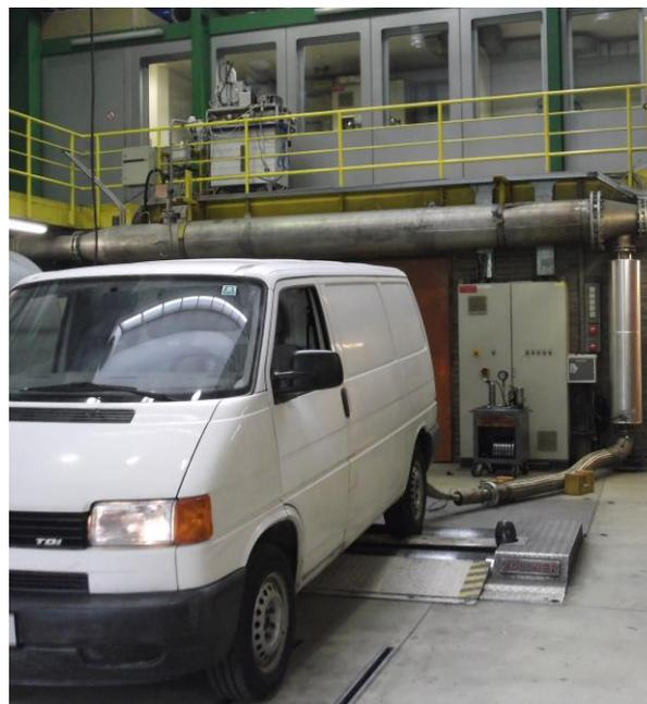
Fig. 1 A diesel van particle emissions test laboratory in “Institute for Internal Combustion Engines and Thermodynamics, Graz University of Technology.
