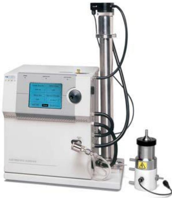
Fig. 2 Particle size distribution measurement device “Series 3080 Electrostatic Classifiers (Courtesy of [www.tsi.com](http://www.tsi.com))”.
