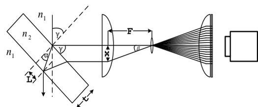
**Fig. 1** Schematic diagrams: transmitting and receiving parts of the optical train.
