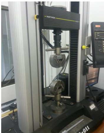
Fig. 8 Tensile testing of the specimens
