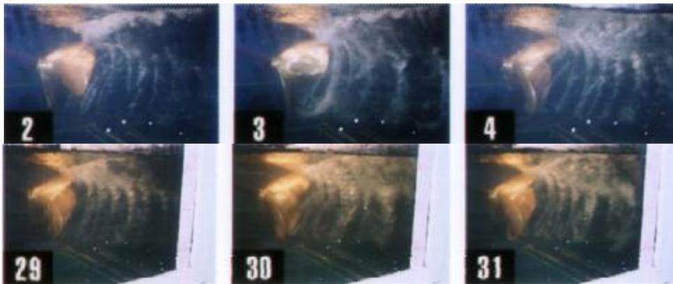
**Figure 17.** Illustration of propeller cavitation type B3-30-50 Velocity 800 rpm. (Tank Test)
