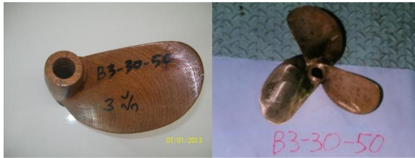
**Figure 13.** Illustration of propeller Model and Propeller casting Type B3-30-50 (New Design)
