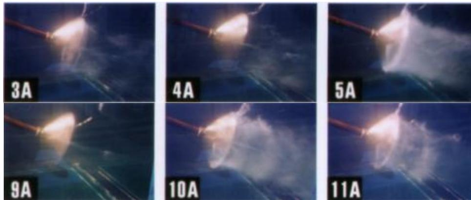
**Figure 14.** Illustration of propeller cavitation type B3-30-35 Velocity 600 rpm. (Tank Test)
