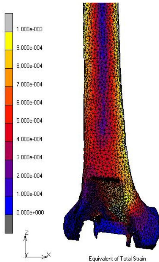
Fig. 7 Show the strain distribution on distal cortex under stair-climbing condition.
