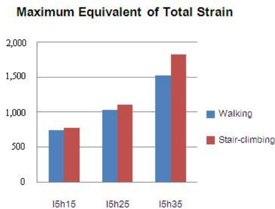
Fig. 6 Show the maximum equivalent of total strain at the anterior notch on distal cortex under walking and stair-climbing condition.
