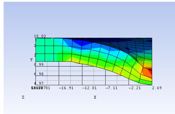
Fig. 5 Section of backup plate showing the indentation after ballistic impact process
