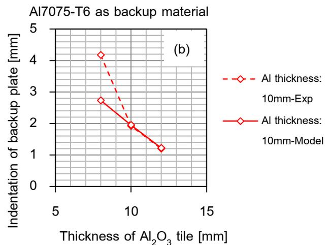
Fig. 6 Validation between numerical and experimental results (a) 4340steel is the backup material (b) Al7075-T6 is the backup material
