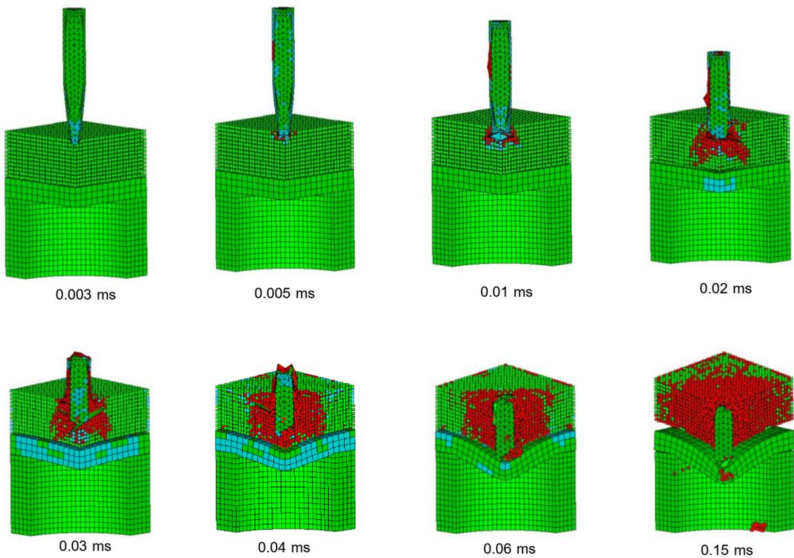
Fig. 3 Chronology of the impact process for the case 9 as indicated in Table. 1
