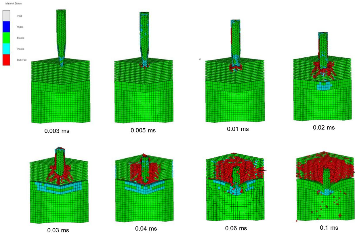
Fig. 2 Chronology of the impact process for the case 3 as indicated in Table. 1
