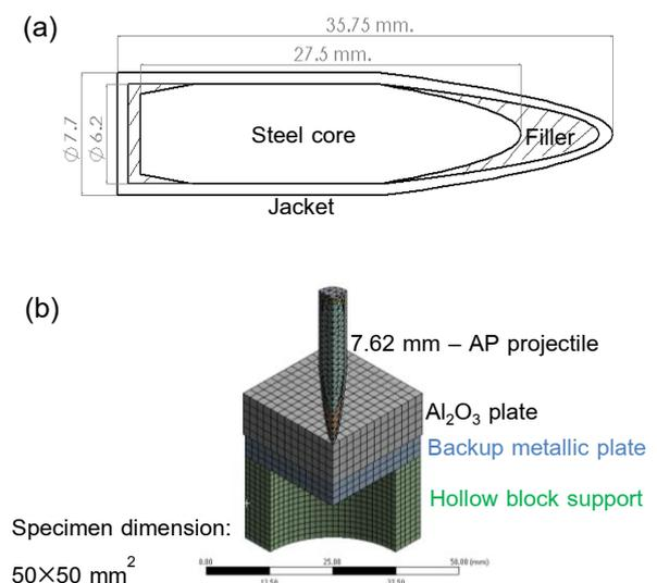
Fig.1 Model construction (a) the dimension of 7.62 mm-AP (0.3 Caliber AP) projectile including internal steel core (b) a quarter model including projectile and specimen
