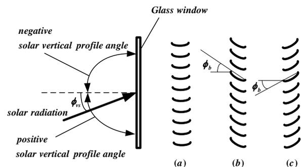
Fig. 5 Glass window and vertical venetian blind with slat setting at 0 angle, positive angle and negative angle.
