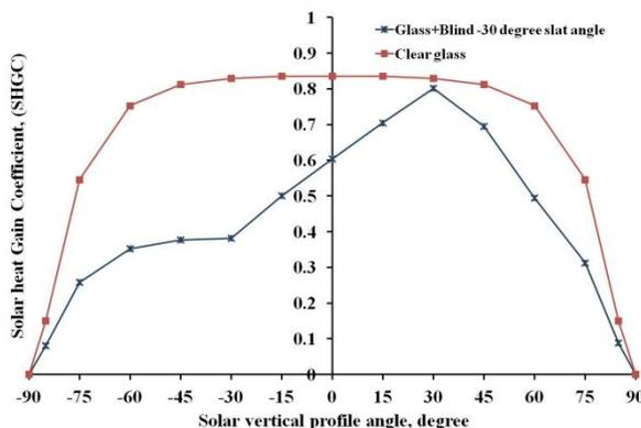
Fig. 8 Variations of the SHGC for a single pane clear glass window and a clear glass window with vertical venetian blind installed with slat angle setting at -30 degree.
