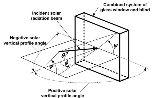
Fig. 1 The combined system of glass window and blind with the incident solar radiation.
