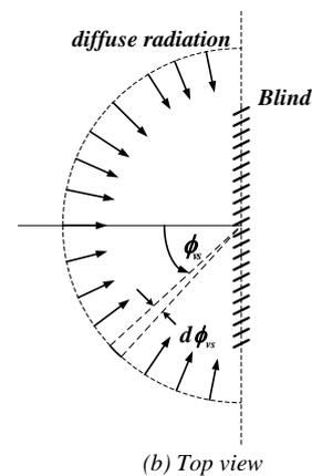
Fig. 4 Distribution of diffuse radiation on the vertical venetian blind.
