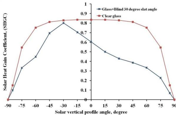
Fig. 7 Variations of the SHGC for a single pane clear glass window and a clear glass window with vertical venetian blind installed with slat angle setting at 30 degree.
