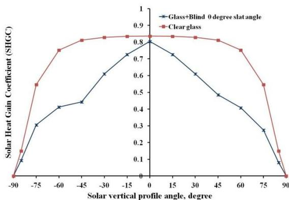
Fig. 6 Variations of the SHGC for a single pane clear glass window and a clear glass window with vertical venetian blind installed with slat angle setting at 0 degree.
