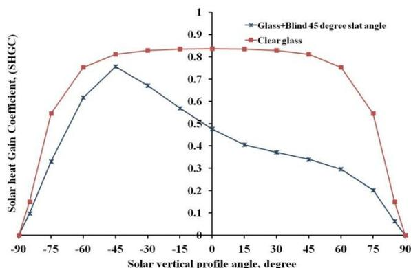
Fig. 9 Variations of the SHGC for a single pane clear glass window and a clear glass window with vertical venetian blind installed with slat angle setting at 45 degree.
