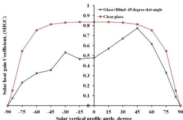
Fig. 10 Variations of the SHGC for a single pane clear glass window and a clear glass window with vertical venetian blind installed with slat angle setting at -45 degree.
