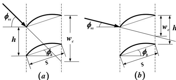
Fig. 2 Curved slat vertical blind at different solar vertical profile angle seen in the horizontal plane.
