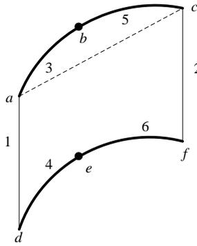
Fig. 3 Six surface closed enclosure formed by two consecutive slats.
