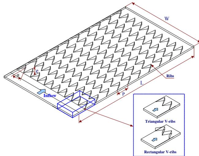
Fig. 2. Test section with rectangular and triangular wavy baffles.
