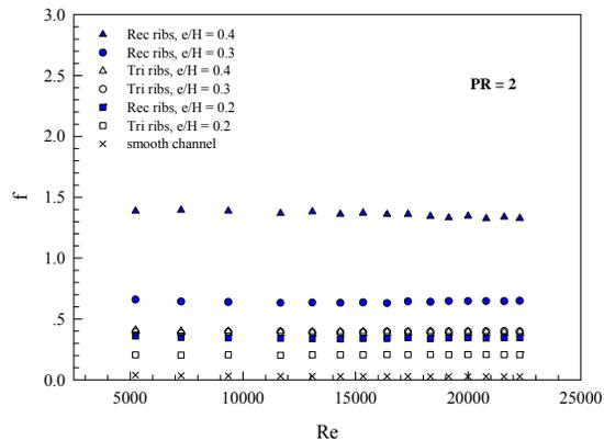
Fig. 5. Variation of friction factor with Reynolds number for various  $e/H$  values.
