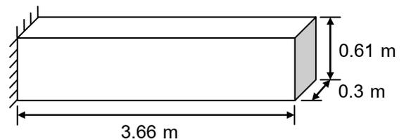
Fig. 7 Geometry of a cantilever beam
