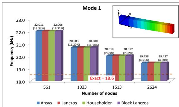
Fig. 8 Comparison of mode frequency values for mode 1 (first bending in *x* direction)
