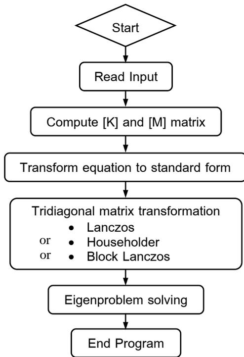
Fig. 1 Procedure of FEM free vibration analysis
