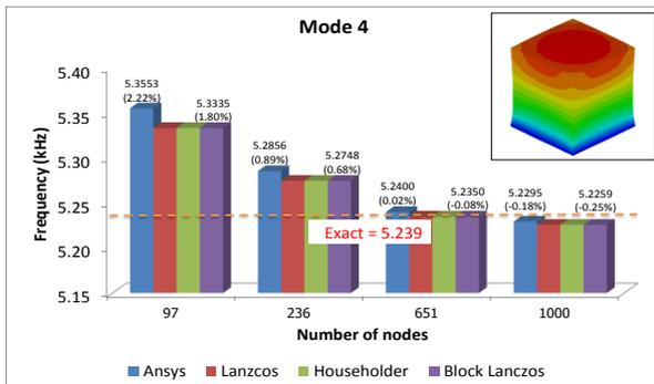
Fig. 5 Comparison of mode frequency values for mode 4 (longitudinal mode)
