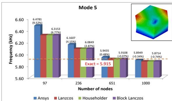
Fig. 6 Comparison of mode frequency values for mode 5 (swaying mode)
