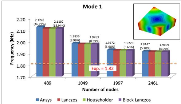
Fig. 12 Comparison of mode frequency values for mode 1 (twist mode)
