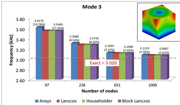
Fig. 4 Comparison of mode frequency values for mode 3 (torsion mode)
