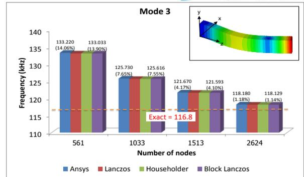
Fig. 10 Comparison of mode frequency values for mode 3 (second bending in *x* direction)
