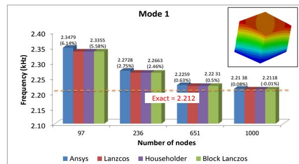
Fig. 3 Comparison of mode frequency values for mode 1 (swaying mode). The values above the columns are mode frequencies computed and differences with the exact solution are shown in parentheses.
