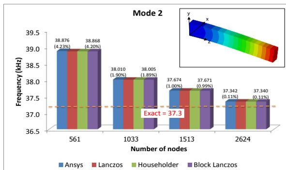
Fig. 9 Comparison of mode frequency values for mode 2 (first bending in *y* direction)
