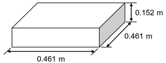
Fig. 11 Geometry of an anvil
