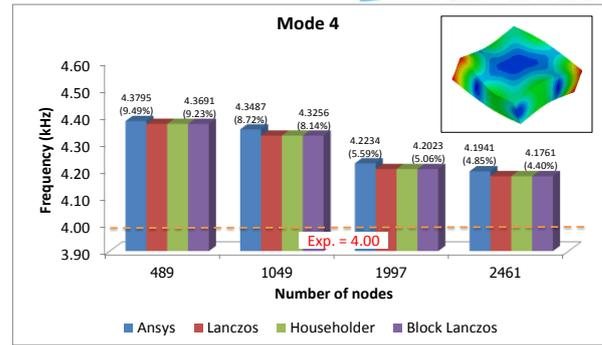
Fig. 15 Comparison of mode frequency values for mode 4 (in-plane shear mode)
