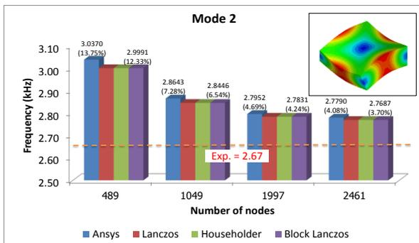
Fig. 13 Comparison of mode frequency values for mode 2 (saddle mode)
