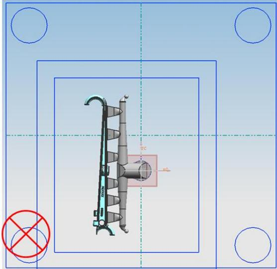
Fig. 3 Layout of part and gating system when placed at vertical position
