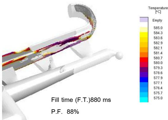
Fig. 6 Non distributed flow pattern when the part and gating system is higher position at 90°
