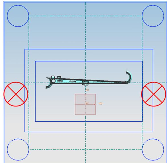
Fig. 2 Layout of part and gating system when placed at horizontal position
