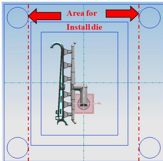
Fig. 5 Layout of part and gating system when move the part and gating system to higher position
