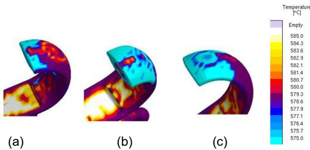
Fig. 8 Temperature distribution on the casting at cavity fully filled (F.T. 1050 ms, P.F. 100%) at (a)  $55^{\circ}$  (b)  $65^{\circ}$  and (c)  $35^{\circ}$  rotation angle.
