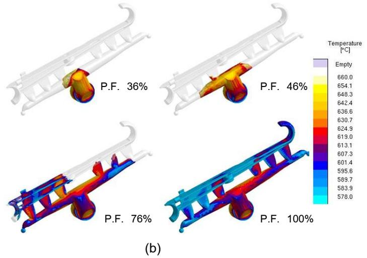
Fig. 4 Shape of Gating system designs and temperature distribution during the filling of (a) Tangential gate (b) Multiple fan gates
