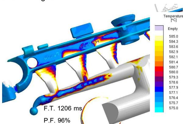
Fig. 9 At melt speed of 0.8 m/s complete solidification take place at the ingate area and casting part
