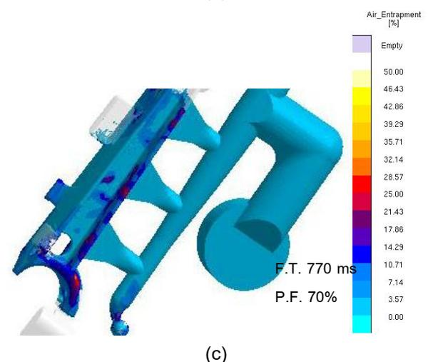
Fig. 10 Air entrapment in the cavity at different melt speed of (a) 2 m/s , (b) 1 m/s, and (c) 0.8 m/s, respectively.
