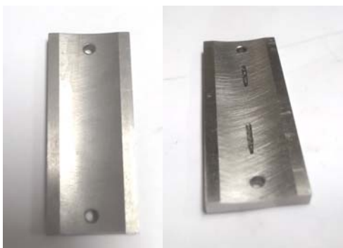
Fig. 2 Cylinder Liner (Before testing : Left, After testing : Right)
