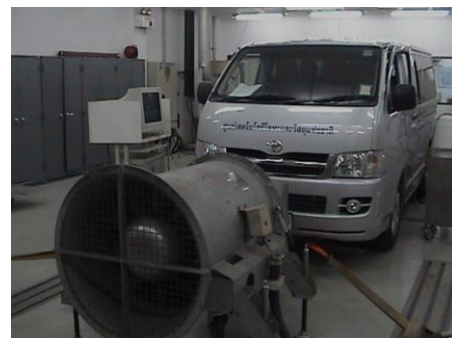
Fig.2 Performance and Emission Test Setup
