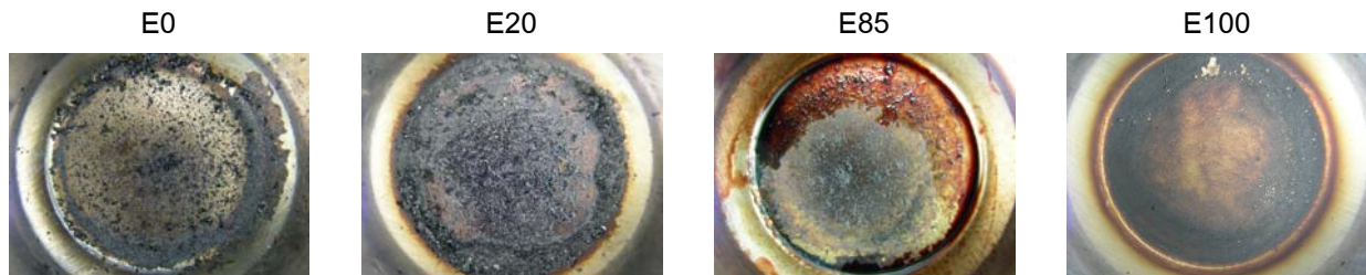
Fig. 1 Photograph of fuel deposits at surface temperature 200 °C for 10 hours test time
