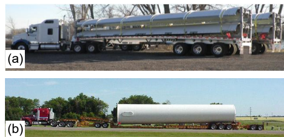
Fig. 4 Transportation of tower components [8]
