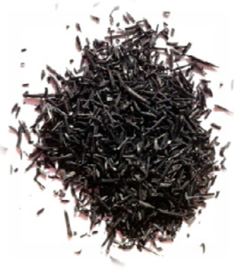
Fig. 3 Rice husk char adsorbent, 0.5-1.0 mm.
