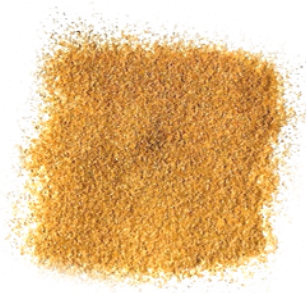
Fig. 2 Rice husk feedstock, 0.125-0.250 mm.
