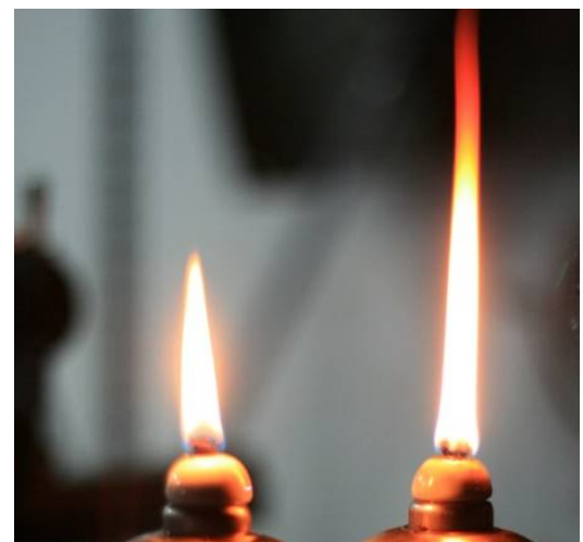
Fig. 3 Biodiesel (left) and diesel (right) diffusion flame by conventional digital camera.
