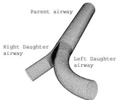
Figure 2 Three-dimensional mesh model of an asymmetric single bifurcation of the central airway
